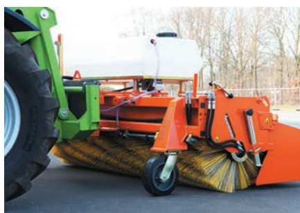
Stable Super-elastic wheels Ø 300 x 90 mm, telehandler attachment
