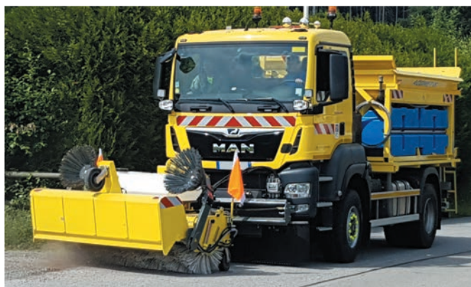
bema 35 Dual PowerMaster with hydraulic lateral movement (collection container opened / free sweeping)
